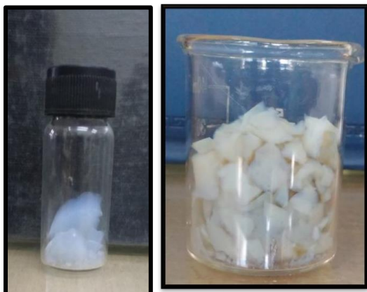
Fig.2: Photographs of a) pure aerogel b) silica aerogel composite nickel nitrate as a additive
